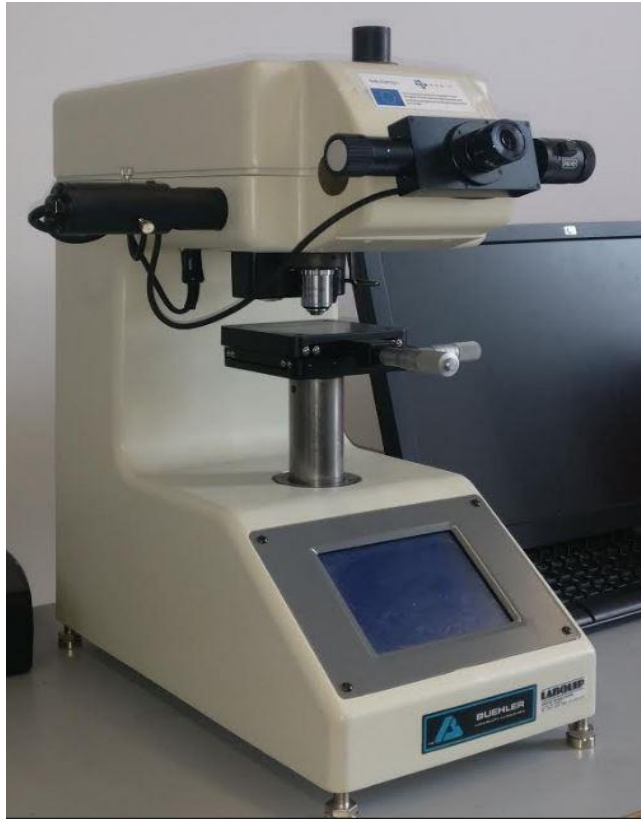
Buehler Micromet® 2100 series microhardness tester
